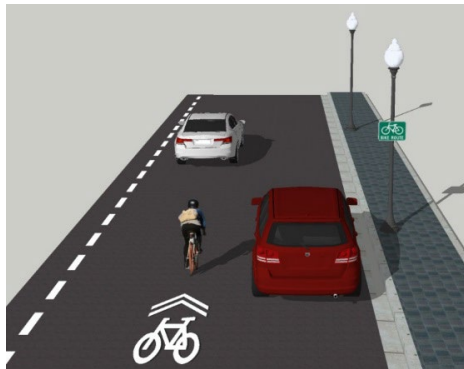
Figure M-8: Standard Class III Bikeway Cross Section
