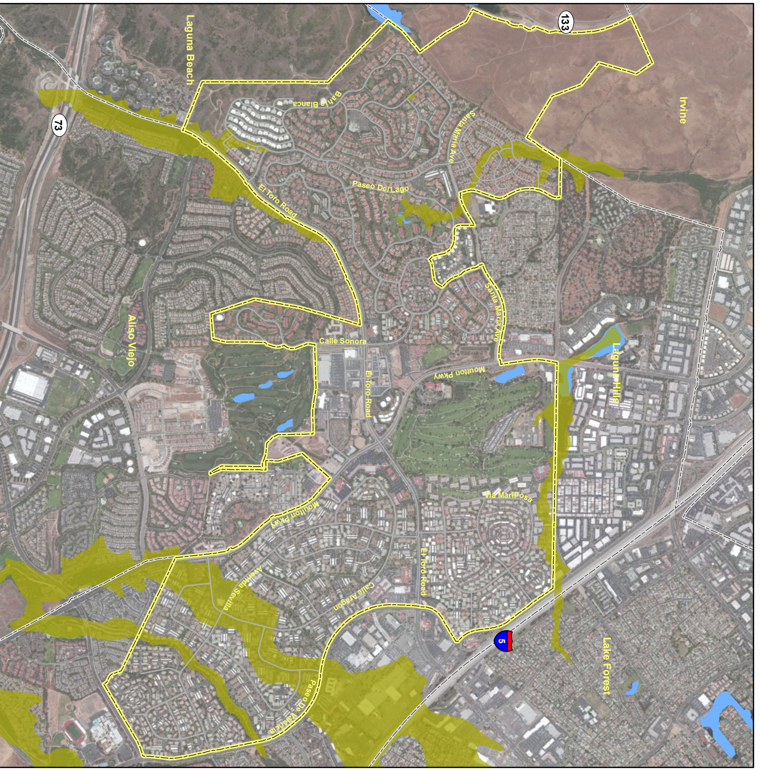
Figure S-5 Liquefaction Hazard Zones
